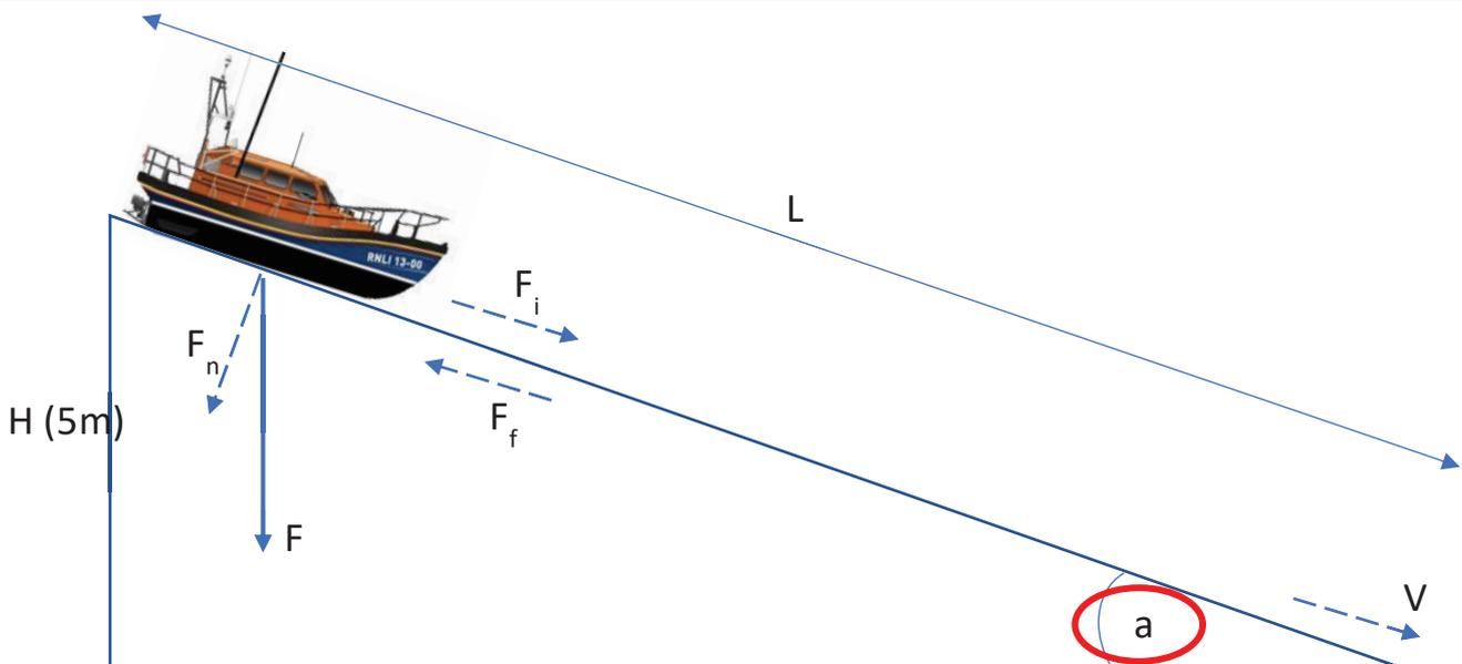
We're looking for the angle  $a$  of the slipway which is shown in the diagram but there are several factors to be included: the height of the station above the water (5m in this case), the forces acting on the lifeboat, the calculated length of the slipway and finally the speed of the lifeboat as it hits the water.
