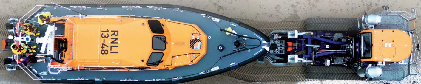
Aerial drone shots of New Quay Shannon class all-weather lifeboat Roy Barker V being launched by SLARS and at sea
