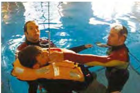
The aim of a retention system (such as a crotch strap) is to improve performance by maintaining the lifejacket around the torso of the user, in order to provide better airway protection.
